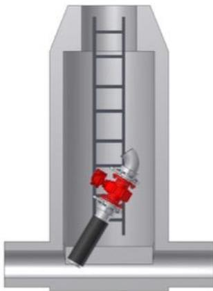
Thread «Portable» in sewer pipe; control with rope
