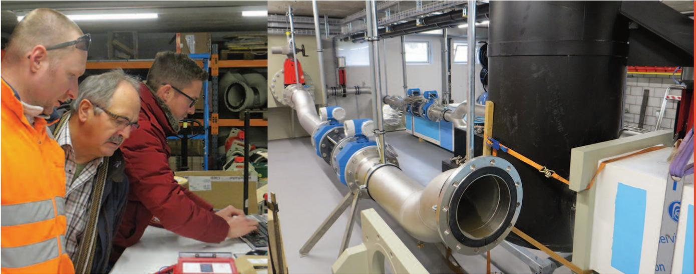
The measurement sections were subjected to extensive tests in the STEBATEC hydraulic lab.
