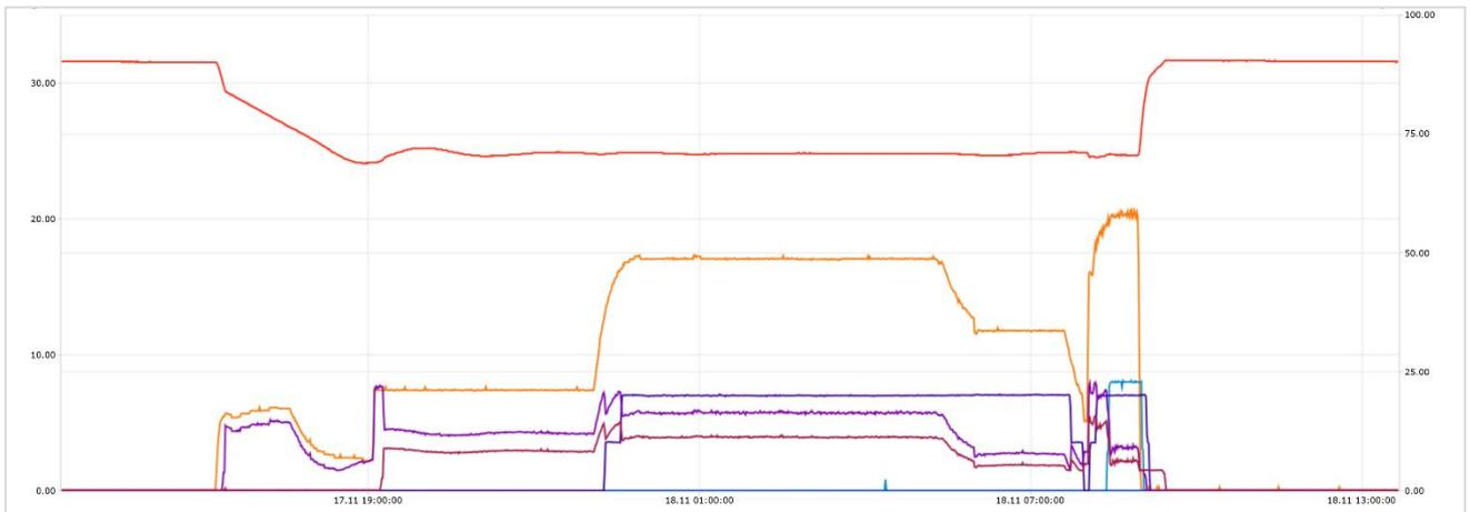
Figure 4: Extract from the data recording of AQUAbella. The red graph represents the level in the water tower (0-100%), yellow the flow rate of all sockets (0-33m<sup>3</sup>/min). The remaining recordings are from the individual sockets.
