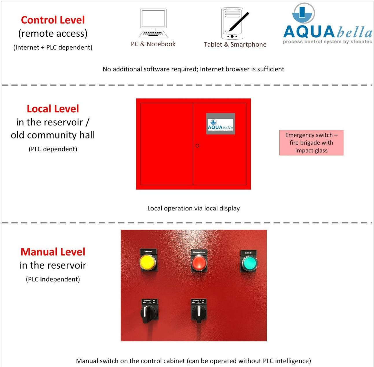
Figure 2: 3-level control concept
